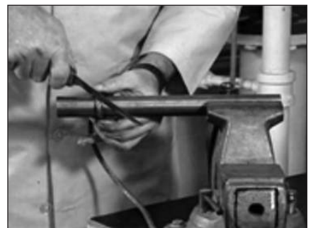
Figure 2b: Skive cut the ring
