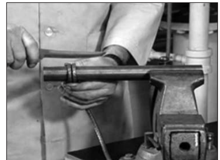
Figure 2a: Mark ring to be cut
