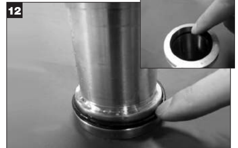
12 Remove O-Ring from sleeve assembly and discard.
