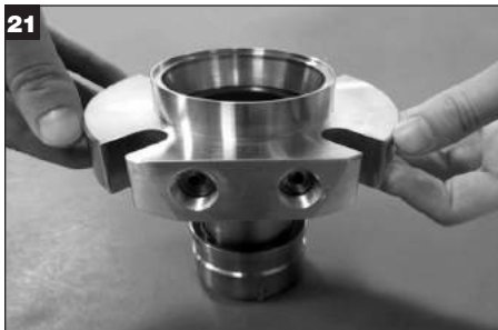
Place gland assembly over sleeve assembly; apply even pressure to gland to ensure faces are seated.
