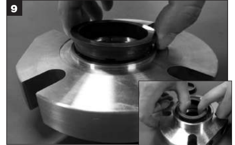
9 Remove both inboard stationary seal rings from gland assembly and discard.
