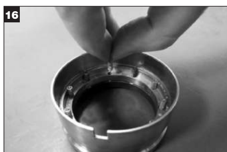
16 Apply a thin film of grease to one end of each spring and install springs in the inboard rotary assembly.
