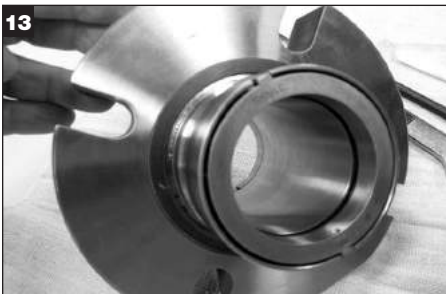
13 Remove gasket from gland assembly and discard.
