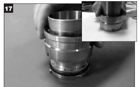
17 Slide rotary holder assembly over sleeve. Align slot in rotary holder assembly with lug in sleeve and compress.
