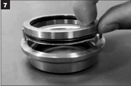
7 Separate spacer from outboard rotary seal ring assembly. Discard rotary seal assembly.
