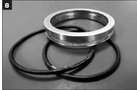
8 Remove two spacer O-Rings and discard.
