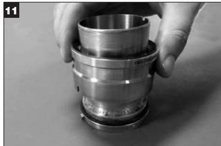
11 Remove the inboard rotary assembly and discard (including springs and O-Ring).
