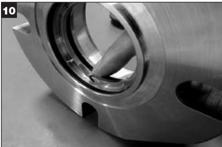
10 Remove both O-Rings from gland assembly and discard.
