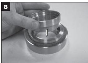
EN Insert stationary holder into gland
