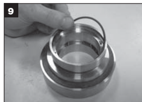
EN Install stationary holder O-Ring
