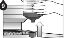
When the selected dispensing period of the Lubri-Cup VG Mini has completed. remove the lubricator from the application.
